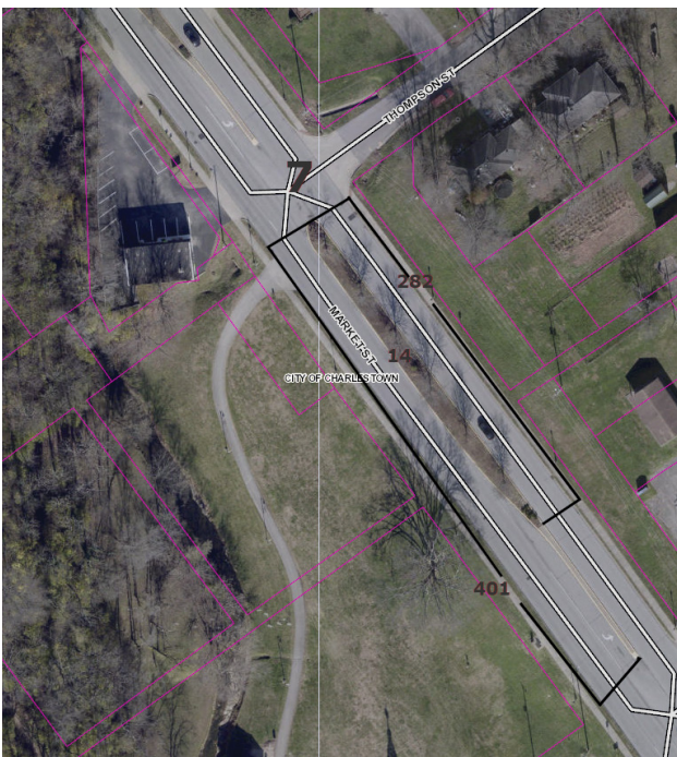
7 (Water Street to Thompson) Length, 401-feet (282-feet of soil); Width, 14-feet at widest point
